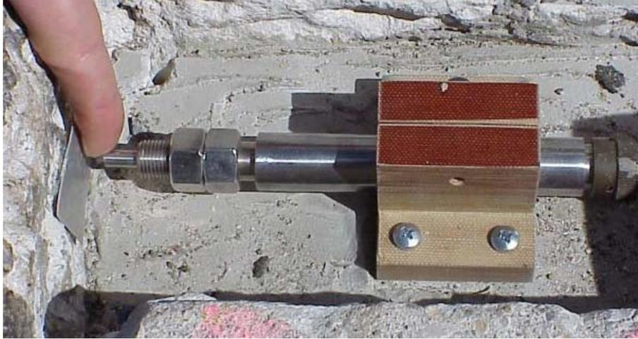
FIGURE 40. JOINT WIDTH MEASUREMENT
