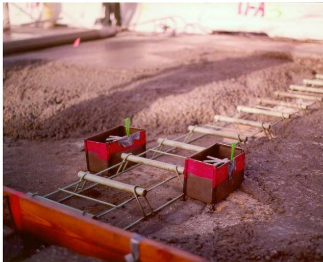
FIGURE 43. STRAIN GAGE PLACEMENT IN THE SLAB
