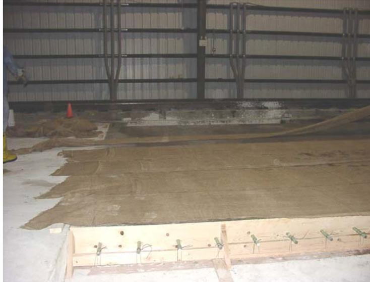
FIGURE 36. PLACEMENT OF BURLAP OVER CONCRETE TEST STRIPS FOR 28-DAY WET CURE
